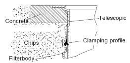
thoroughly coated with the lubricating soap included in the delivery (use no lubrication that is mineral oil based). **Attention:** If the lubricating soap becomes dry and the telescope becomes difficult to move then there is the danger that the sealing ring will be forced out of its recess. Before filling, the sealing ring must be checked once again that it is seated correctly in position. The telescope must be sufficiently embedded and supported that no forces are transferred to the housing.
