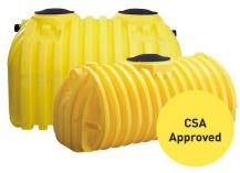
These environmentally safe & seamless one piece tanks are watertight and unaffected by soil chemicals and gases in sewage. Therefore, they are corrosion-resistant. They come pre-plumbed with PVC inlet and outlet assemblies and fit both 4" SCH 40 and SDR35 piping. Unlike the Bruiser, they cannot be used as pump out tanks and must be kept full at all times, or as soon as possible after pump out.
