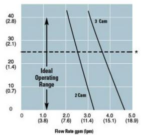
\*Continuous Duty Max Pressure For No Switch 3 Cam Models
