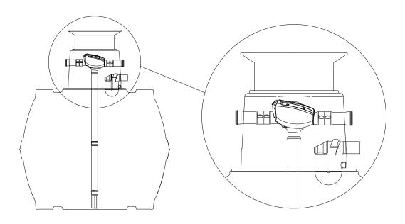
Insert the filter, prepared with the inflow Calming Foot, in the tank.
