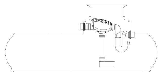
Insert the filter, prepared with the inflow Calming foot, in the tank.
