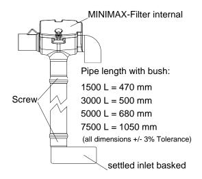
Following this a 250 mm long inlet pipe and an overflow siphon are pushed in to the Platin underground tank until the end stop position as shown in the adjacent depiction.
