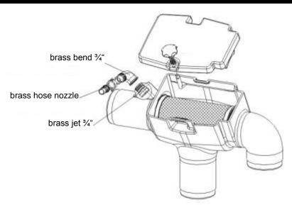
The brass jet ¾" is to be inserted in the provided aperture at the inlet side of the filter housing and fixed with the brass bend from the outside. Afterwards the brass hose nozzle is to be screwed on with a union nut and connected with the hose (provided by customer). The hose is conducted through the empty conduit to the pump and linked with the pressure line on the pressure side after a cut-off cock.
