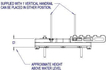
IT IS POSSIBLE TO ALTER THE VARIABLE WIDTH BEYOND STANDARD BY CUTTING THE PIPES TO DECREASE THE WIDTH OR REPLACING THE PIPES WITH LONGER PIPES (1.5" SCHED 80) TO INCREASE THE WIDTH
