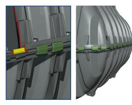
Thanks to the additional ribbing, the Carat S underground tank suffers no significant warping even under extreme loads. Therefore, the Carat S underground tank is suitable for vehicle loading up to a total weight of 3.5 tonnes, groundwater-stable up to the middle of the tank and can be installed with an earth covering up to 47". Additionally, the encircling H profile acts as a convenient carry handle for transport and as a tread when fitting the tank dome.
