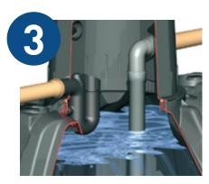
Dirt particles that are lighter than water (e.g. pollen) settle on the water surface as a floating layer which is automatically removed when the tanks is full and overflows to the drainage system through the Overflow Siphon Assembly inside the tank. So, regular overflowing of the tank is important for consistent water quality.
