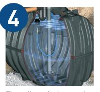
The collected rainwater is extracted from the tank using a Floating Suction Assembly that always draws water from just below the surface (approx. 4" or 10 cm) as this is the location of the optimum water quality. The GRAF Rainwater Harvesting System brilliant design and highly effective - simply providing the best water quality possible prior to treatment.
