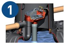
The rainwater is first cleaned by a patented Filter System(s). The cleaned water runs into the tank and dirt particles are rinsed into the sewer system with a small amount of water. BARR offers different filter systems for every installation situation.
