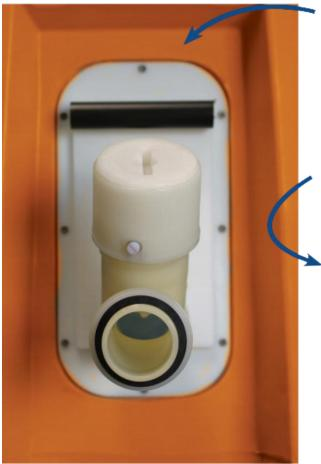
2" reusable discharge valve contains a piercing ring which taps into the bag as the valve is screwed into place. Attach the reusable 2" valve and tap into the liner in one easy step. The slopped bottom assures complete drainage.
