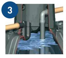
Dirt particles that are lighter than water (e.g. pollen) settle on the water surface as a floating layer which is automatically removed when the tanks is full and overflows to the drainage system through the Overflow Siphon Assembly inside the tank. So, regular overflowing of the tank is important for consistent water quality.
