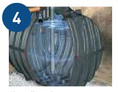
The collected rainwater is extracted from the tank using a Floating Suction Assembly that always draws water from just below the surface (approx. 4" or 10 cm) as this is the location of the optimum water quality. The GRAF Rainwater Harvesting System – brilliant design and highly effective – simply providing the best water quality possible prior to treatment.
