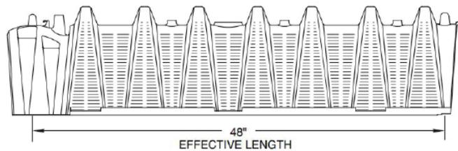
The MultiPort end cap fits on either end of the Quick4 Equalizer 36 Chamber and allows multiple piping options. Six molded-in inlets/outlets allow for maximum piping flexibility. Patent-pending tear-out seals on inlet ports provide a tight fit to the pipe, eliminating pipe fittings and making looping ends easy.
