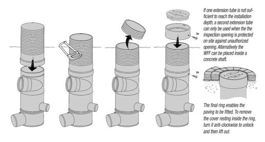
• The vortex filter is not a closed system, it must not be flooded for a longer period of time. In loamy soil, provide drainage underneath the filter, or seal the joints of the filter housing from the outside with a suitable sealant before installation. In case of non-observance seepage water may enter the filter from the outside.
