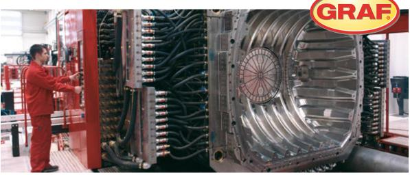
The GRAF Carat S tank range is produced using a method that is as yet unique for tanks of this size. The injection compression process gives the products an incomparable stability – all Carat S underground tanks are suitable for vehicle loading and can be installed in groundwater up to the middle of the tanks. Additionally, the new method guarantees that the components will fit; a result that cannot be achieved with conventional production methods.
