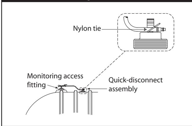
**4.5.3.** The quick-disconnect assembly must not be connected to the service fitting when pressure testing the primary tank. Keep the nylon tie in place.
