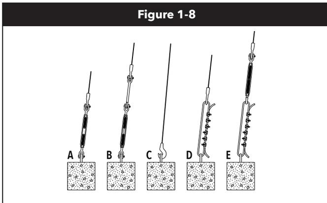
**1.3.6.3.7.** If using a wire rope, refer to recommendations of wire rope manufacturer and supplier, and follow accepted industry standards when selecting, using, attaching or connecting wire rope. Most wire rope suppliers provide rigging educational courses, including free online options. See **Figure 1-8** and **Figure 1-9**.
