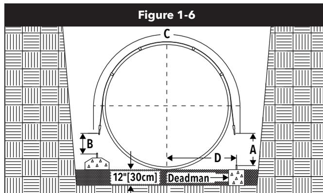
**NOTE:** If a D-ring/D-ring strap is used on a 4-foot-diameter tank, the anchor point must be 3 inches [8 cm] below the top of the bedding.
