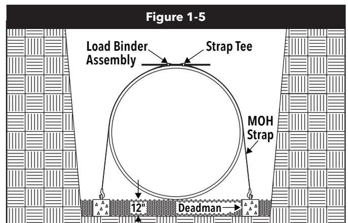
**1.3.6.2.11.** MOH anchor straps are to be installed in the following way:
