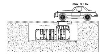
Cover heights with cast or HGV-bearing telescopic dome shaft
