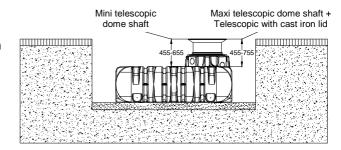
Maximum coverage heights with extension and telescopic dome shaft.
