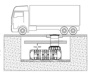
Coverage heights on installation in groundwater – the hatched area specifies the permissible immersion depth for the tank.
