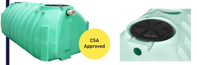
This tough low profile tank, introduced to the North American market in 2012, can be used as a CSA approved septic tank, holding tank, pump chamber, or cistern for non-potable water applications such as rainwater collection, stormwater management or fire protection. Heavy duty and rotationally-molded in one piece, it providesleak-free reliability. Furthermore, they come with the baffle wall and fitting holes already in-place, reducing installation time and effort.
