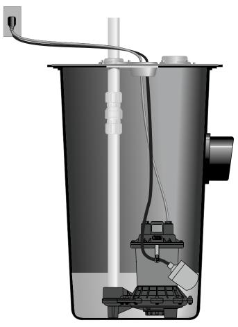
Figure 2: ME40 Typical Installation
