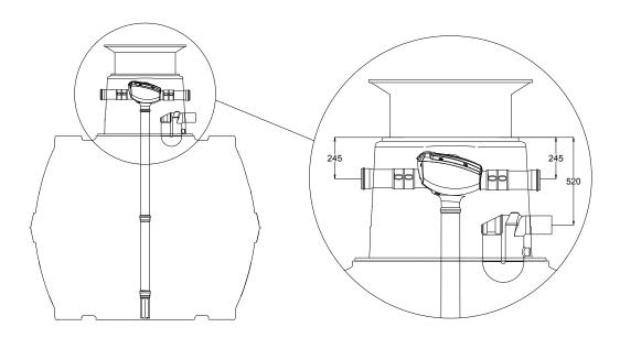
5.6 Installation of inflow pipe and overflow siphon
