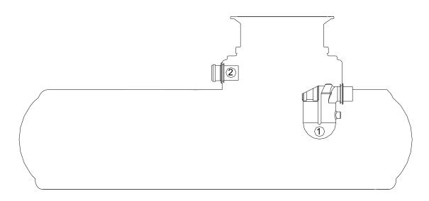
Insert the overflow siphon in the lower seal till block.
