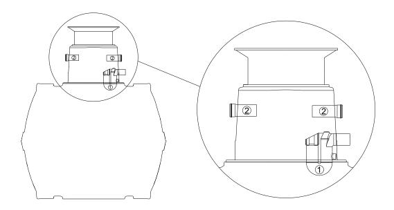
Insert the overflow siphon in the lower seal till block.
