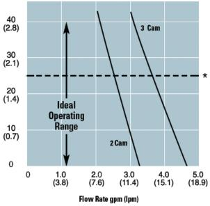
\*Continuous Duty Max Pressure For No Switch 3 Cam Models
